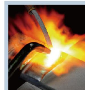
Oxy-Acetylene Flame Welding System
