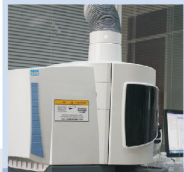
Inductively Coupled Plasma Optical Emission Spectrometer(ICP-OES)
